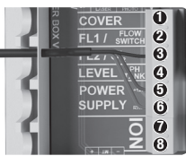
Chlorine probe detector FL2 (rotameter) ③ black ⑤ brown ⑥ blue
