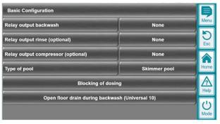
Assignment of the relay outputs used
