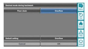
An info text (at the bottom of the menu) summarizes the result of the current configuration, e.g. "During a backwash, suction is taken out of the gutter tank"
