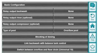
Assignment of the relay outputs used
