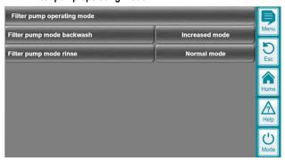
· Choice of filter pump speed for backwash and rinse
