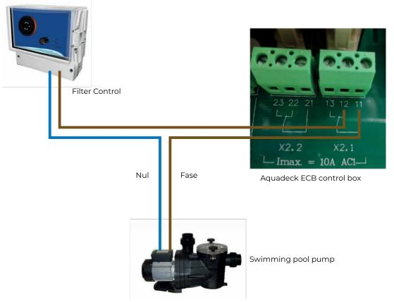
Select option 3 in menu 31 of the ECB control box (installation in service)
