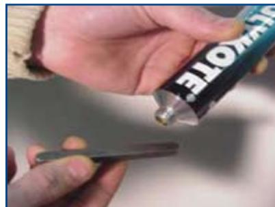
Grease key and fit in the drive motor.
