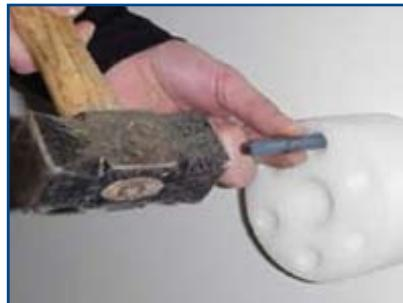
Use a punch to drive tap bolts completely into the hole.
