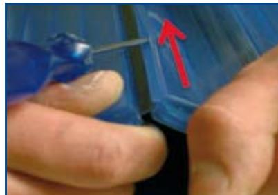
Place a thin, flat screwdriver between the hook and the groove and slide it toward the other end of the slat so the hook comes loose from the groove.
