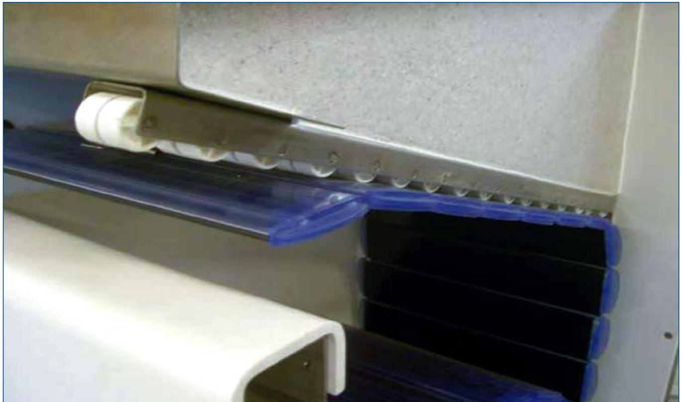
Always place the guide rollers between two straps to prevent snagging or damage of the straps.
