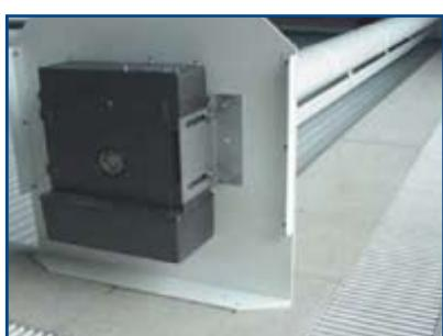
Mount the drive motor using the motor bracket.
