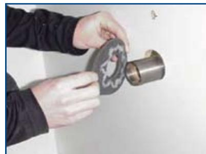
Fit gasket with sealant in motor well.
