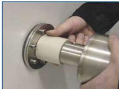
Slide out drive shaft, fit spacer bush in between and secure with M10 bolt.
