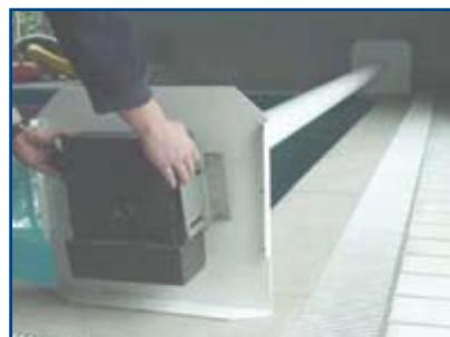
Fit drive motor and check that the tube turns smoothly.
