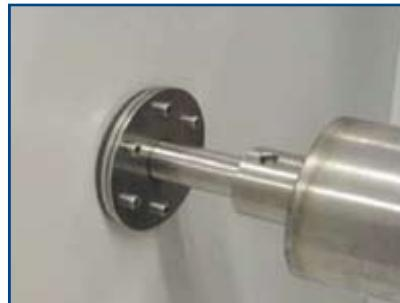
Slide drive shaft into coupling bush of tube.
