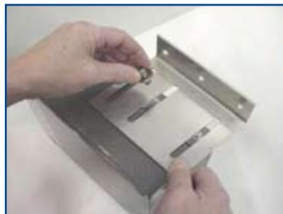
Fit motor bracket on motor.
