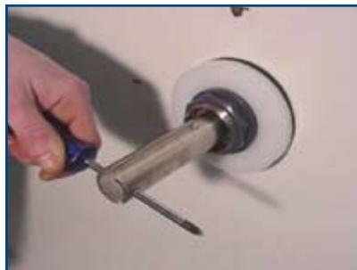
**TIP!** Use drilled hole at keyway to move shaft.
