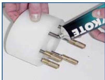
**TIP!** Applying a bit of grease
