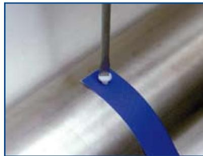
Attach the straps to the winding tube.
