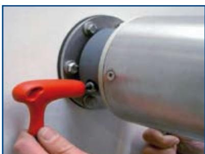
Secure the bolt with the crown nut.
