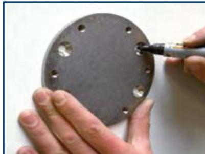
Position pre-assembled element on bearing side and mark 4x countersunk holes.
