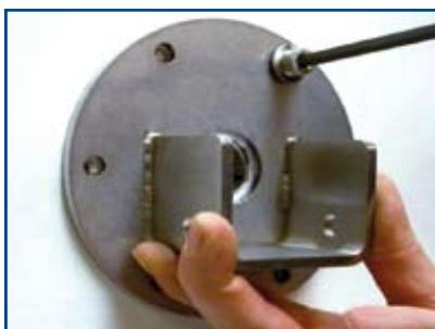
Secure the motor flange using the short M8 bolts with neoprene washers.
