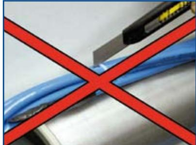
Do not cut the control cable loose with a blade.
