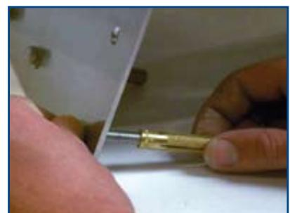
First thread the WAKO plugs onto the bolts (with washers).
