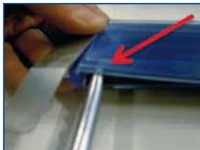
Open the groove of the slat with a screwdriver and slide the bracket over the slat.
