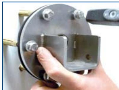
Position the motor flange and drive in the bolts until they are flush with the flange.
