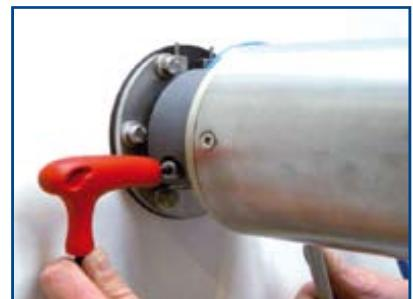
Secure the bolt with the crown nut.
