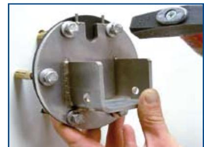
Position the motor flange and tap the bolts until they are flush with the flange.
