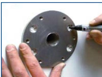
Position pre-assembled element on motor side and mark 4x countersunk holes.
