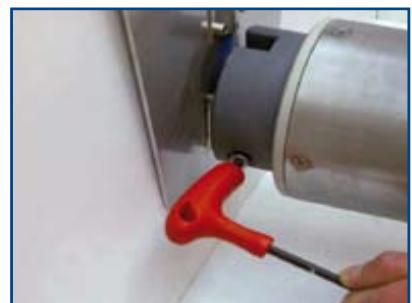
Fit the bolt and secure it with the crown nut.
