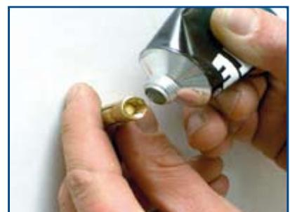
**TIPP!** A bit of grease inside of the WAKO plug prevents the entry of dust that makes the bolts difficult to turn.
