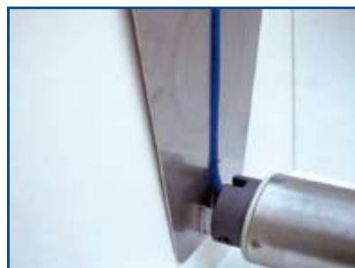
Slide the winding tube over the U-profile.
