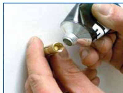
**TIP!** A bit of grease inside of the WAKO plug prevents the entry of dust that makes the bolts difficult to turn.
