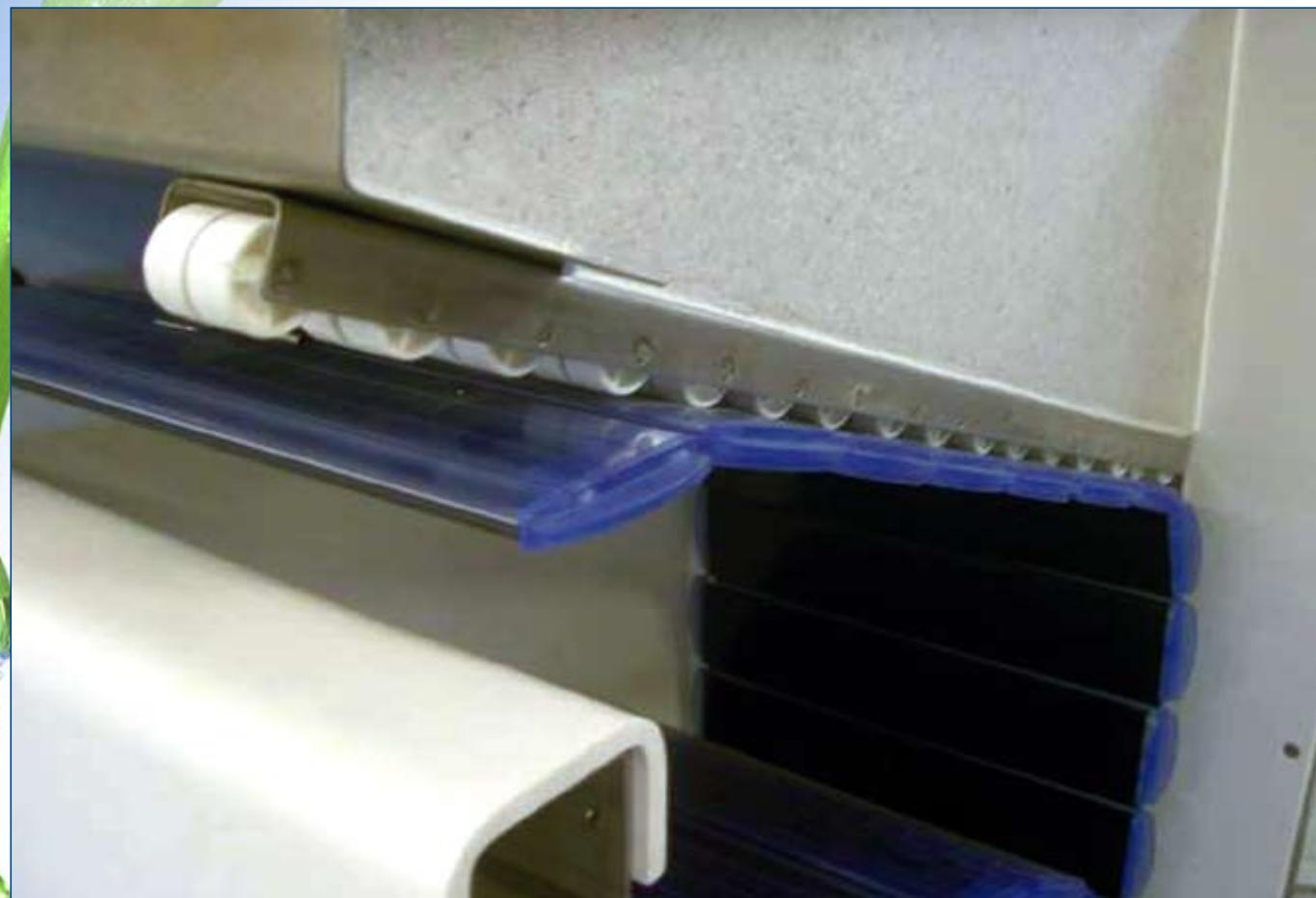
Always place the guide rollers between two straps to prevent snagging or damage of the straps.
