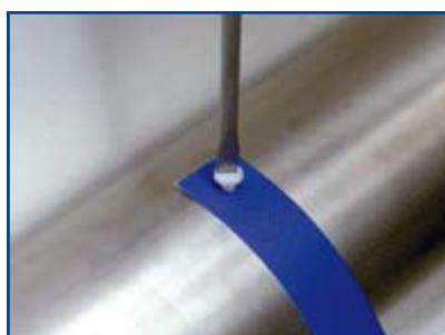
Attach the straps to the winding tube.
